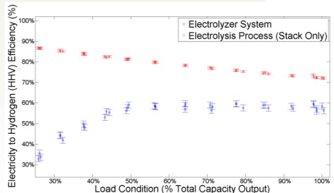
Stack and system efficiency at part load for 60kW PEM Electrolyzer
