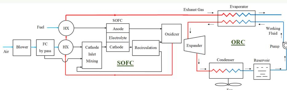
Figure 2: Configuration for SOFC-ORC System
