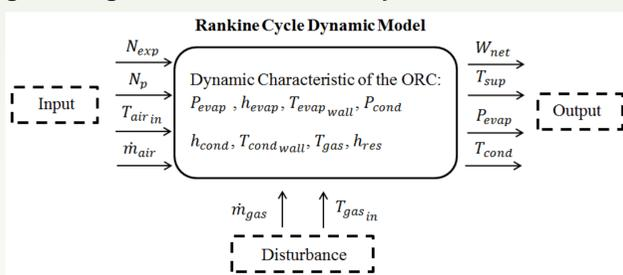
Figure 1: Information Diagram of the ORC Simulation Model
