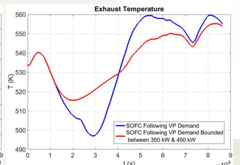
Figure 8: SOFC Exhaust Gas Temperature
