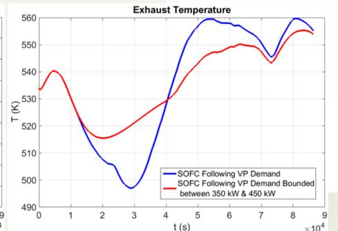
Figure 8: SOFC Exhaust Gas Temperature
