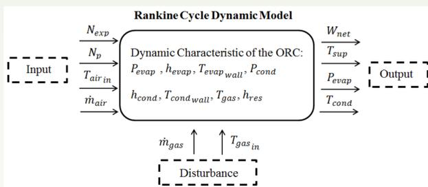
Figure 1: Information Diagram of the ORC Simulation Model
