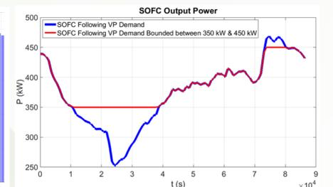
Figure 6: SOFC Output Power
