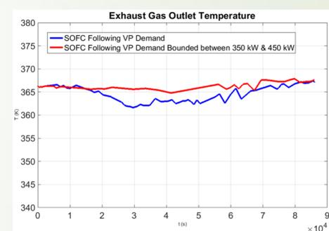
Figure 10: Exhaust Gas Outlet Temperature after Transferring Heat in ORC
